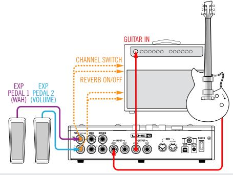
\*IMPORTANT! Connect EXT AMP 1/2 only to amplifiers that utilize "short-tosleeve" footswitch inputs. Connecting to any other sort of input could cause permanent damage to both your amp and HX Effects hardware! If you're not sure if your amp has short-to-sleeve inputs, contact the manufacturer.
