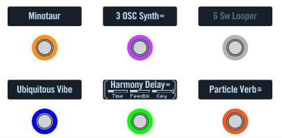
TIPS: Use the Global Settings > Footswitches > Stomp Mode option to configure either all six of the left switches as stomp switches ("6 Swtch"), versus the left two switches as Bank/Preset/Snapshot Up-Down and 4 stomp switches (4 Swtch").
