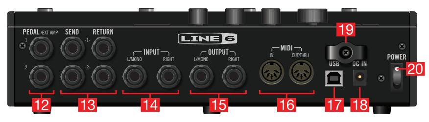
**12. PEDAL/EXT AMP 1-2** Two expression pedals can be connected to the HX Effects device and assigned to adjust a wide variety of parameters. When adding blocks within the Signal Flow view, EXP 1 is automatically assigned to control and bypass Wah, Pitch Wham, or Poly Wham blocks, and EXP 2 is automatically assigned to control Volume and Pan blocks, making them ready for use with your connected expression pedal(s). See <u>"Assigning a Controller"</u>
