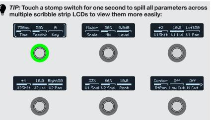
Touch the desired footswitch to select its parameters and then turn knobs 1-3 to adjust them. If a block has more than 18 parameters, press  $\triangleright$  to access more parameters. When finished, touch a switch for one second (or press  $\widehat{m}$ ) to exit.
