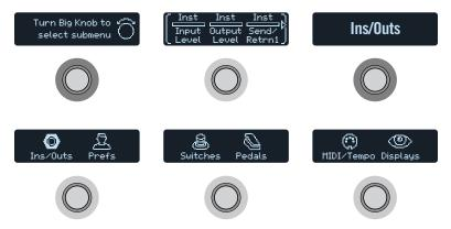
**3.** Turn the Big Knob to select one of the six submenus. If necessary, press ▷ to view more parameters.
