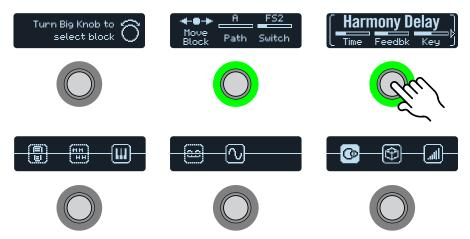
Touch FS2 for block moving, routing, and footswitch assignment.
