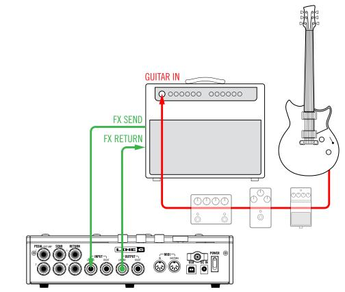
NOTE: The effects loops on most amplifiers run at instrument level. If your amp's effects loop happens to run at line level, you should set the inputs and outputs of your HX Effects device to line level as well. See <u>"Setting Proper Levels"</u>
